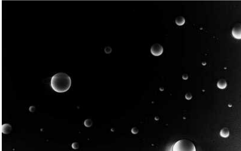
Left: Light microscopy of organic-inorganic hybrid photovoltaic cell structure with surface defects (2012)
